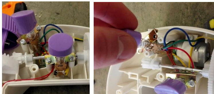
Figure 2.3 (left): Power and lamp switches mechanically attached to the casing. Figure 2.4 (right): ADC team member Rowan removing the power switch from the sewing machine.
